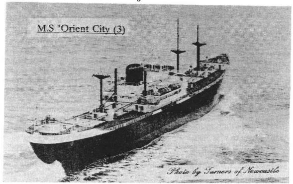
M.V."Orient City" (3) was built in 1960 by William Doxford & Sons Ltd of Sunderland for the Reardon Smith Line. It was a closed shelter deck vessel of 10,300 gross registered tonnage with a 1,072 nominal horse power engine. The engine was a Doxford 5 cylinder, type LB, 700 mm bore, electric power was supplied by three Bellis and Morcom diesel generators.
