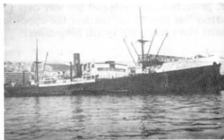
s.s. "Quebec City". Completed 1927. Launched at Wm. Gray Yard, W. Hartlepool. Length 414' 7". Breadth 54' 3". (2nd of 11 vessels (Gray) 1927/30.)
