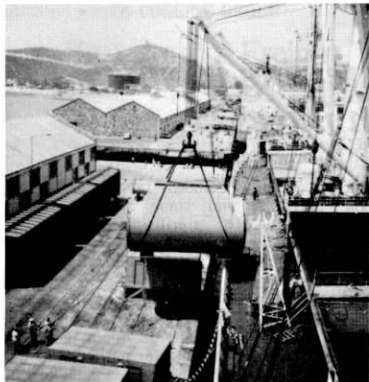
m.v. "Amparo" discharging 95.5 ts./68 ts. lifts, using ship's gear.
